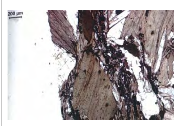
Figure 13: S_2 Parallel Shear Surfaces Marked by Granules of Staurolite and Small Parallel Flakes of Biotite Truncating Earlier Biotite Porphyroblasts, Direction Sense of Movement is Indicated by Dragging of Basal Cleavage of One Biotite Porphyroblast, Near Sini Pahar, Northern Part of the Area
