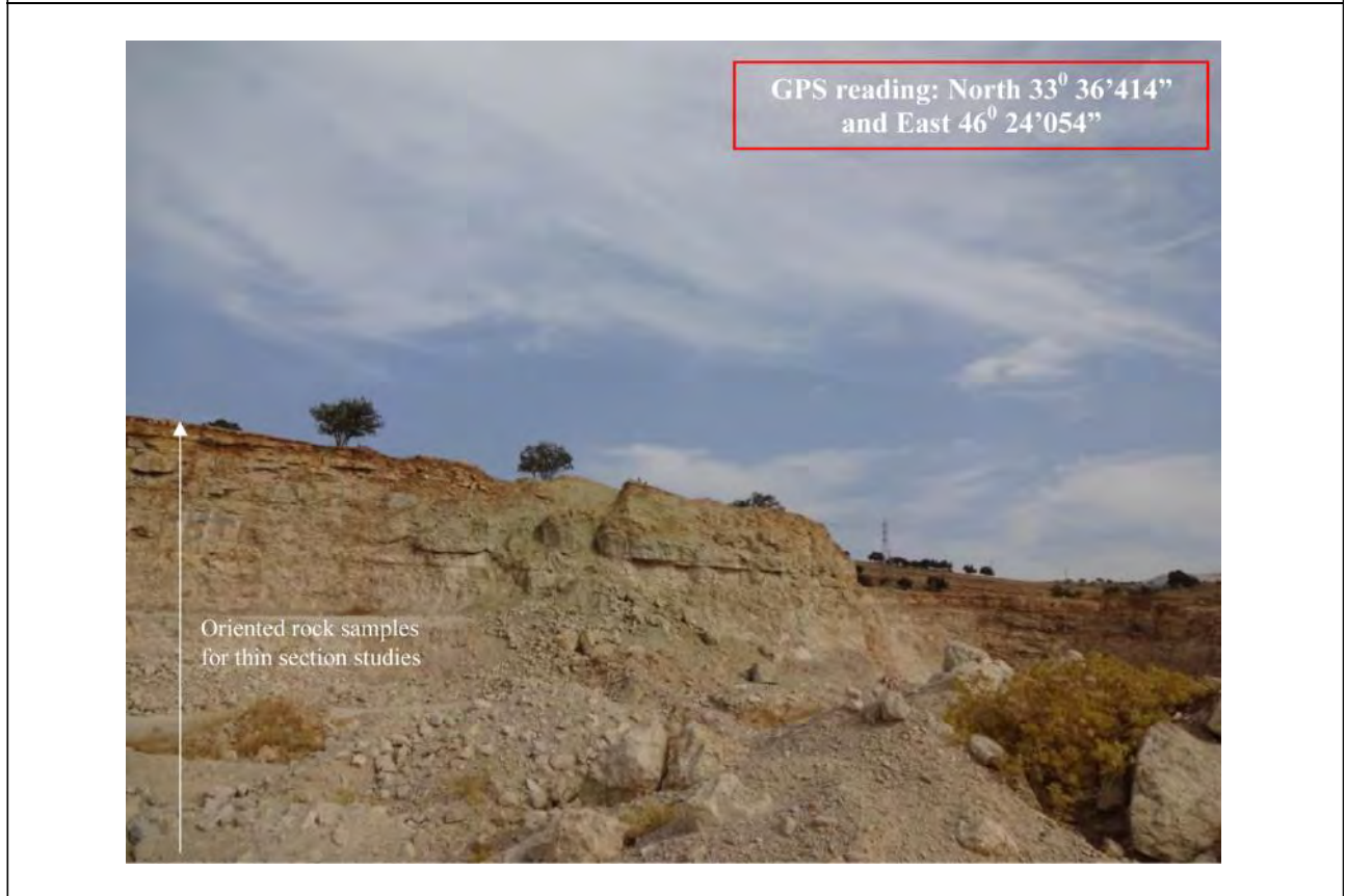
Figure 4: Shows Limestone Cuttings in Sarableh Open Cast Mine, In this 28 Fresh Oriented Representative Samples Collected for Thin Section Studies
