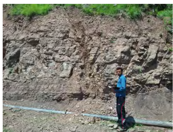
Photo 7: Photograph Shows Soft and Friable Sandstone of Dhok Pathan Formation near Holar. Coordinates 73°37'40" E, 33°36'06" N
