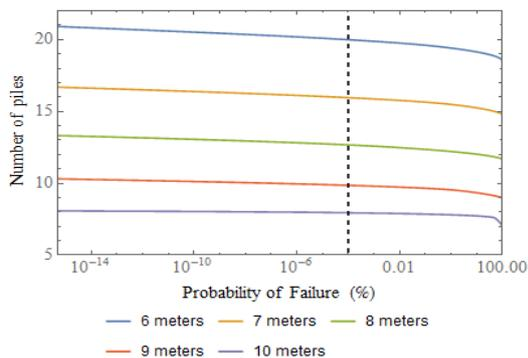
Figure 6. Probability of failure ( $P_f$ ) x number of piles at different depths. Method of Décourt and Quaresma.
