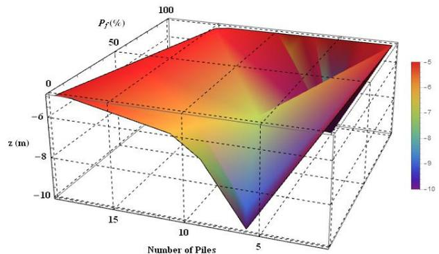
Figure 3. Probability of failure ( $P_f$ ) x laying height ( $z$ ) x number of piles. Aoki and Velloso's method (1975). (b) method of Décourt and Quaresma (1978).
