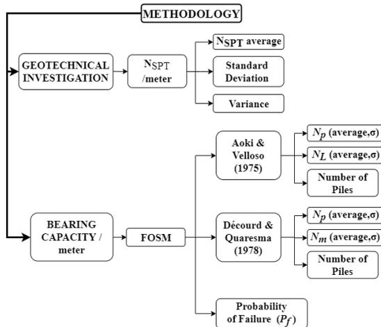
Figure 1. Methodology of the application of the FOSM method on foundation bearing capacity.
