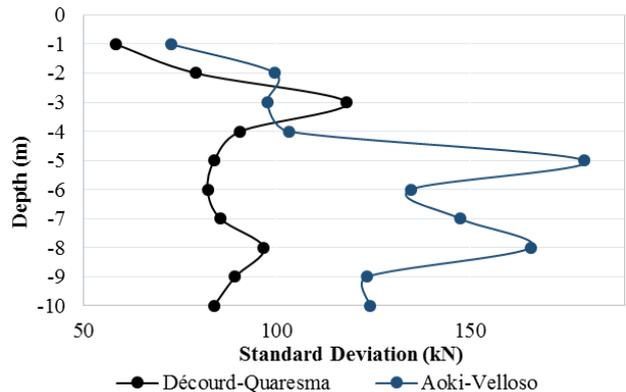
Figure 8. Contribution of the  $N_{SPT}$  for the calculation of the bearing capacity variance at  $z = 10m$ . Décourt & Quaresma Method.
