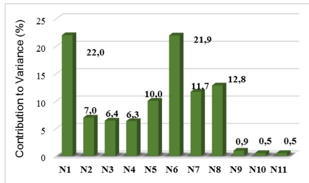
Figure 7. Contribution of the  $N_{SPT}$  for the calculation of the bearing capacity variance at  $z = 10m$ . Aoki & Velloso Method.
