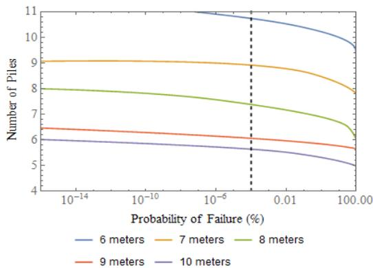
Figure 5. Probability of failure ( $P_f$ ) x number of piles at different depths. Method of Aoki Velloso.
