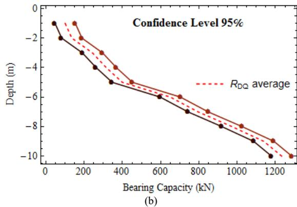
Figure 10. Bearing capacity reliability of the Aoki-Velloso method. a) confidence level of 90%; b) confidence level of 95%.
