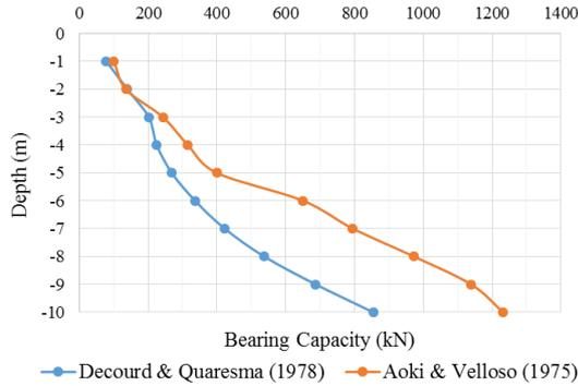
Figure 2. Bearing capacity using mean NSPT values.
