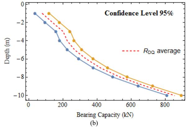
Figure 11. Bearing capacity reliability of the Décour-Quaresma method. a) confidence level of 90%; b) confidence level of 95%.
