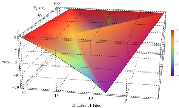
Figure 4. Probability of failure ( $P_f$ ) x laying height ( $z$ ) x number of piles. Method of Décourt and Quaresma (1978).
