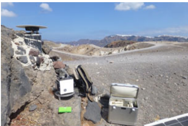
Fig. 3. Gravity/GNSS monitoring station in Nea Kameni in Santorini caldera, Greece, built on a lava outcrop. Gravimeter LaCoste&Romberg-D during observation. One of the young volcanic craters behind the station, and Thira caldera cliffs at the back.
