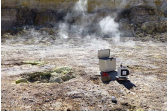
Fig. 7. Gravity measurements at the bottom of the Stefanos crater in Nisyros island. Gas activity in the crater is well visible.
