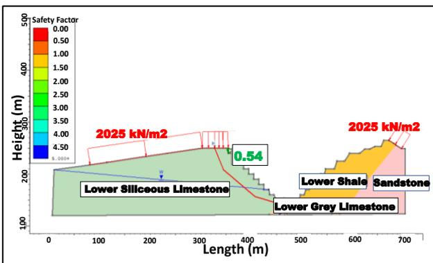
Figure 9. Formation of a critical failure surface at a surcharge dump loading from a distance of 0m from the top of the pit slope [28].
