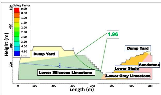
Figure 7. Numerical analysis of critical section in the saturated condition in circular failure.
