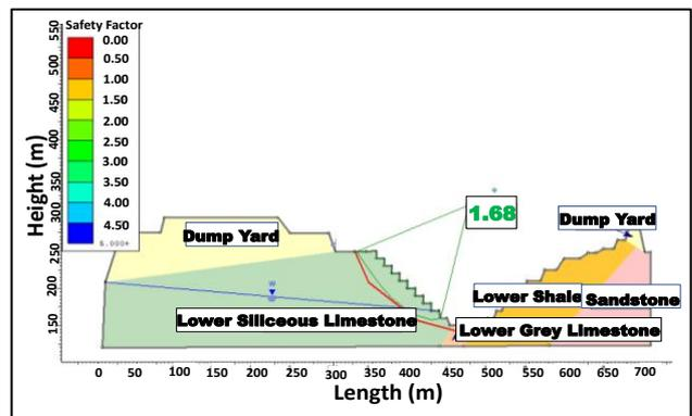
Figure 8. Numerical analysis of critical section in the saturated condition in non-circular failure.
