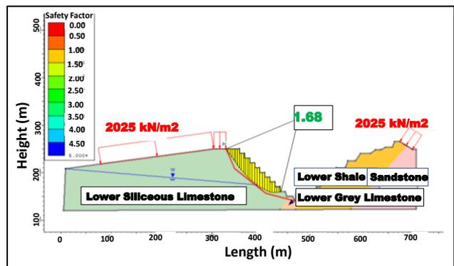
Figure 10. Formation of a critical failure surface at a surcharge dump loading from a distance of 25m from the top of the pit slope [28].
