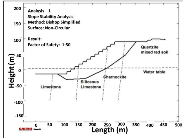
Figure 15. Planned pit slope stability analysis along failure section [29]
