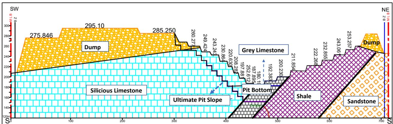
Figure 4. A View of the geological critical section in the mine [28].
