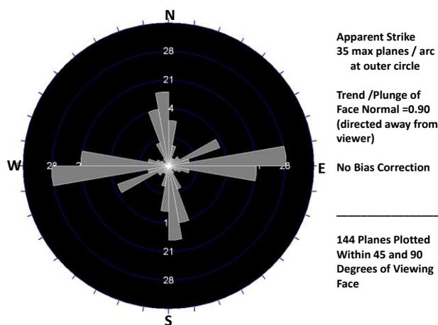
Figure 6. A Rose diagram of all the joints in the limestone mine [28.]
