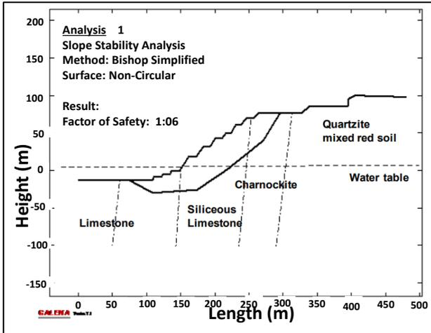
Figure 14. Pit slope stability analysis along failure section [29]
