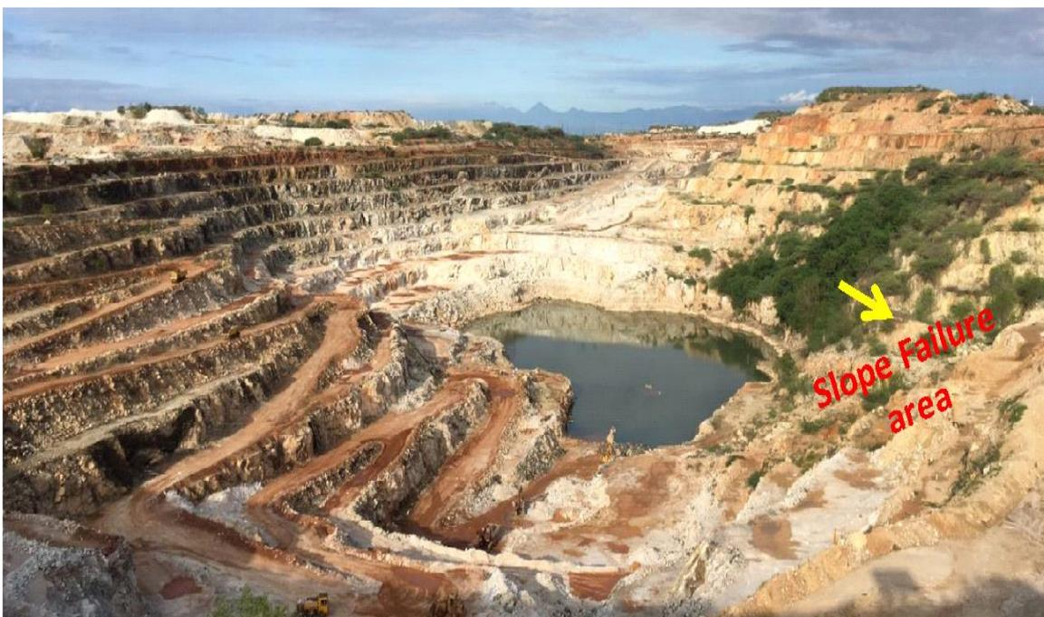
Figure 11. A photograph showing slope failure area in the limestone mine [29].
