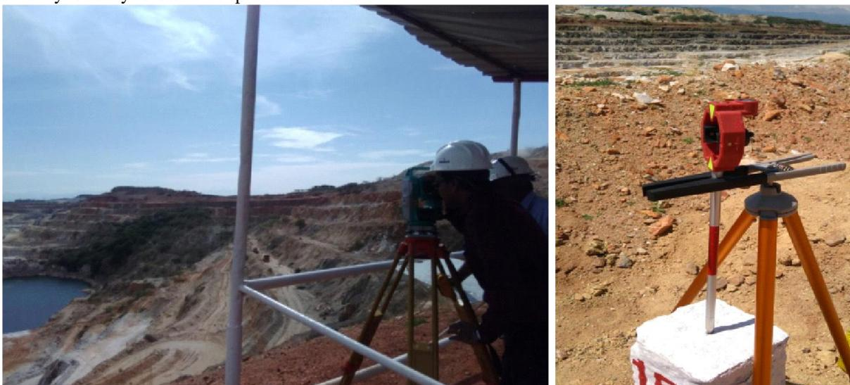
Figure 13. Prism network and monitoring setup in the limestone mine [29]
