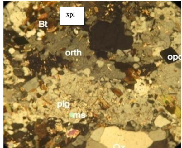
Fig. 22. Photomicrograph of granite (IF25-2) in XPL (x40), musc = muscovite, qz = quartz, plg = plagioclase, fsp = feldspar, bt = biotite, hnb = hornblende, opq = opaque mineral, orth = orthoclase.
