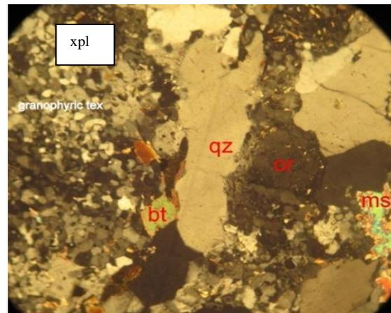
Fig. 23. Photomicrograph of granite-gneiss contact in Tsauni north east (IF 46C) in XPL(x40). Note the elongated quartz porphyroblast at the center between granite and gneiss and the fractured quartz at the right side of the field of view. The granite shows granophytic texture. qz = quartz, bt = biotite, ms = muscovite, or = orthoclase.
