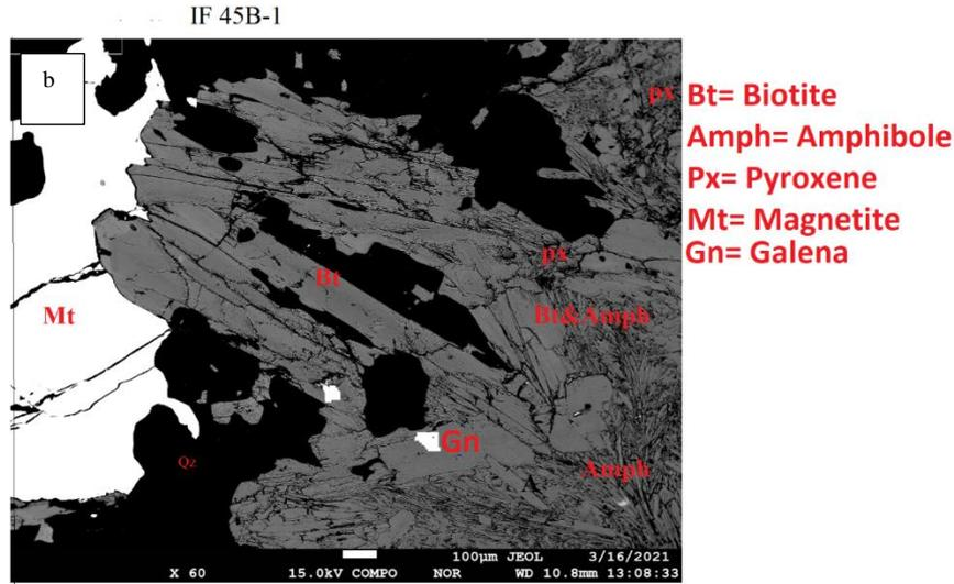
Fig. 27. a–b: BSE images of the typical mineralogy of skarn in the study area.
