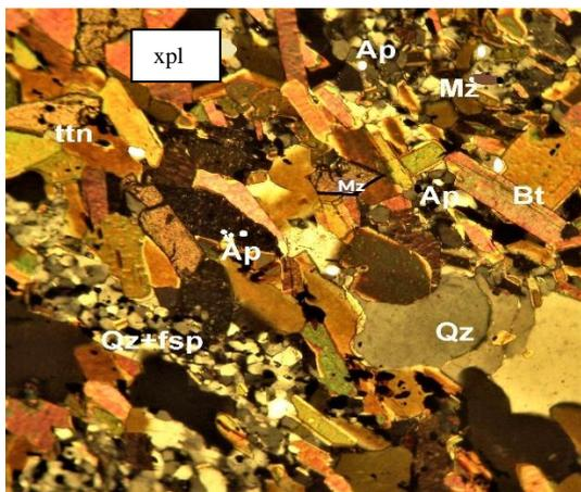
Fig. 21. Photomicrograph of skarn type B (IF 41B-2) in xpl (x40), qz = quartz, fsp = feldspar, bt = biotite, ttn = titanite, mz = monazite, Ap = apatite. Opaque minerals are disseminated.
