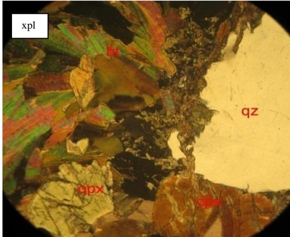
Fig. 19. Photomicrograph of skarn type A (IF 45 B-1) in xpl (x40), qz = quartz, bt = biotite, cpx = clinopyroxene, Amph=amphibole, Ap = apatite, cal = calcite.
