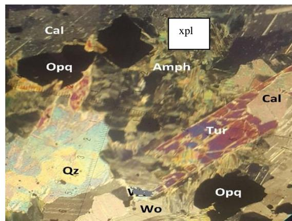
Fig. 18. Photomicrograph of skarn type A (IF 41A) in xpl (x40), qz = quartz, cal = calcite, amph = amphibole, bt = biotite, Tur = Tourmaline, Wo = wollastonite, Opq = opaque mineral.
