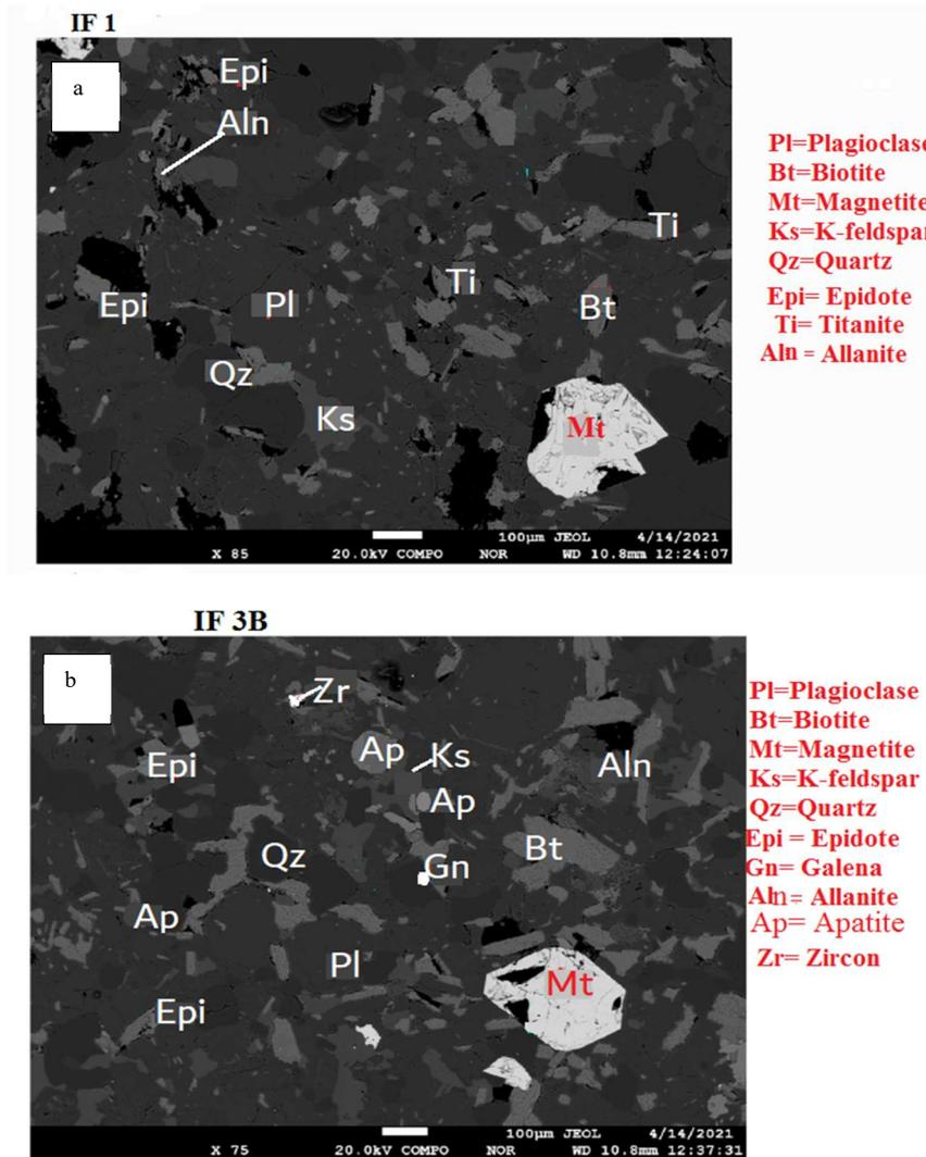
Fig. 25. a–b: BSE images of selected migmatite-gneisses from the study area. Note the sub-euhedral magnetite grains and galena blebs overgrowths on the main mineralogy.
