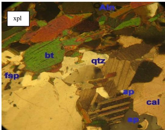
Fig. 20. Photomicrograph of skarn type B in xpl (x40), bt = biotite, qz = quartz, cal = calcite, fsp = feldspar, ap = apatite, Aln = allanite.
