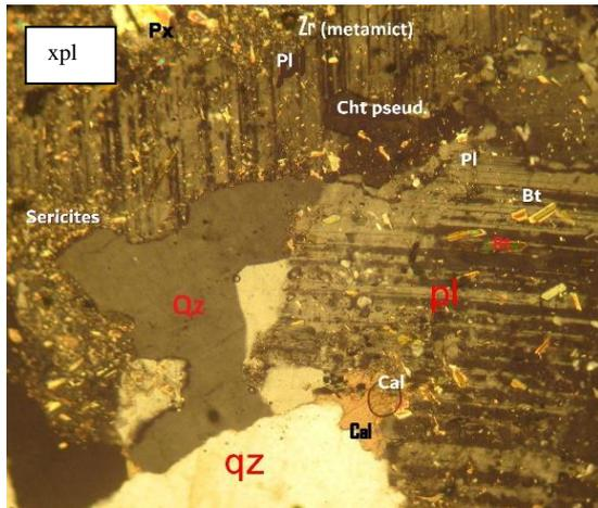
Fig. 16. Photomicrograph of migmatite exposed at Tsauni southeast (IF 5a) in the study area showing pophyroblasts of plagioclase and quartz in xpl (x40), qz = quartz, bt = biotite, cal = calcite, pl = plagioclase. Note the interstitial calcite between plagioclase and quartz at lower right of field of view.
