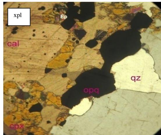
Fig. 17. Photomicrograph of skarn (IF 39 A) in xpl (x40), qz = quartz, cal = calcite, cpx = clinopyroxene, Ep = epidote. Note the primary calcite and zonation of the minerals in the skarn.
