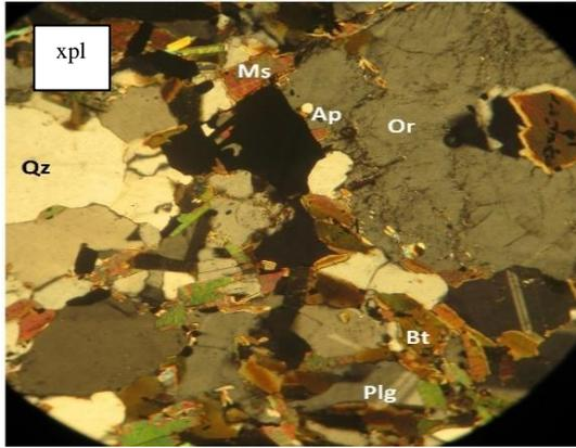
Fig. 15. Photomicrograph of migmatite exposed at Tsauni northeast (IF 42b) in xpl (x40), qz = quartz, bt = biotite, opq = opaque, pl = plagioclase, ap = apatite. Note the porphyroblast of orthoclase that totally replaced the “atoll” plagioclase to the right and biotite foliation.
